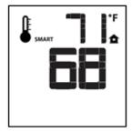
Figure 12: Smart flame function set low.
