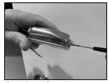
Figure 34: Insert small flat screwdriver.
