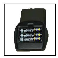
Figure 6: Proflame 2 remote battery compartment.
