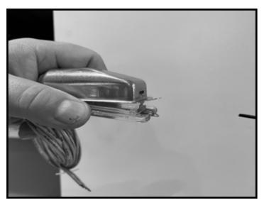
Figure 35: Twist to open glass lens.
