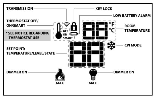
Figure 2: Proflame 2 LCD screen details.
