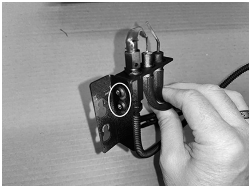
Figure 11: Remove pilot mounting bracket.
