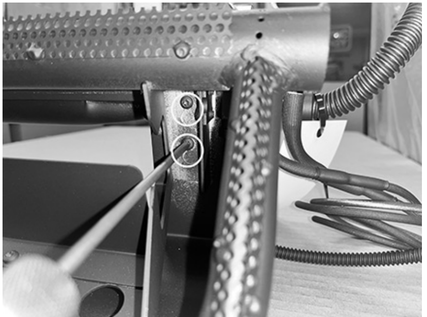
Figure 13: Attach the Unit pilot to the burner tray.
