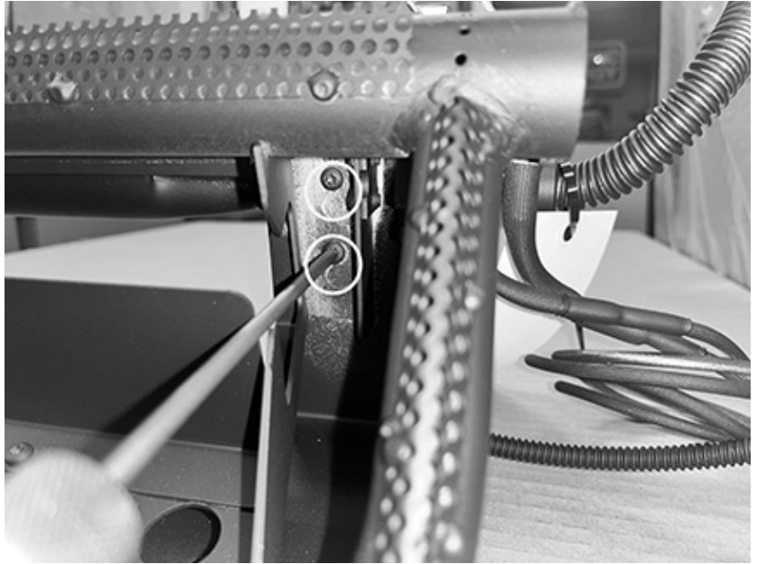
Figure 10: Remove burner pilot.
