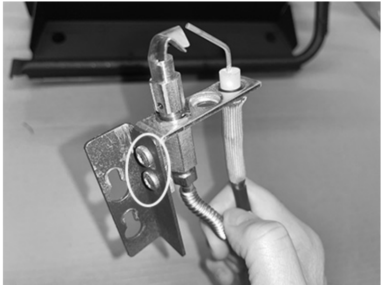
Figure 12: Attach pilot mounting bracket to Unit pilot.
