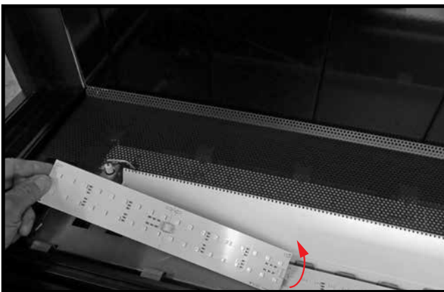
Figure 62: LED strip removal.
