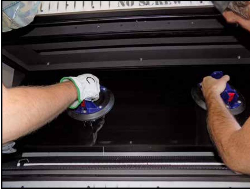
Figure 34: Insert top end of rear black glass plate first.
