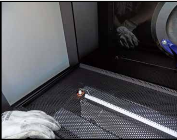
Figure 36: Rear black glass plate in place.
