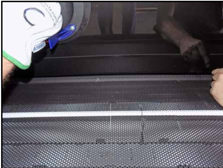
Figure 35: Lift bottom end of black glass over the rear mesh screen.
