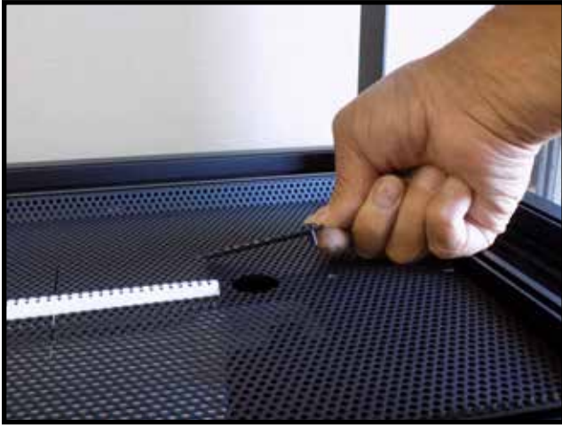
Figure 39: Securing cover plate to burner tray.
