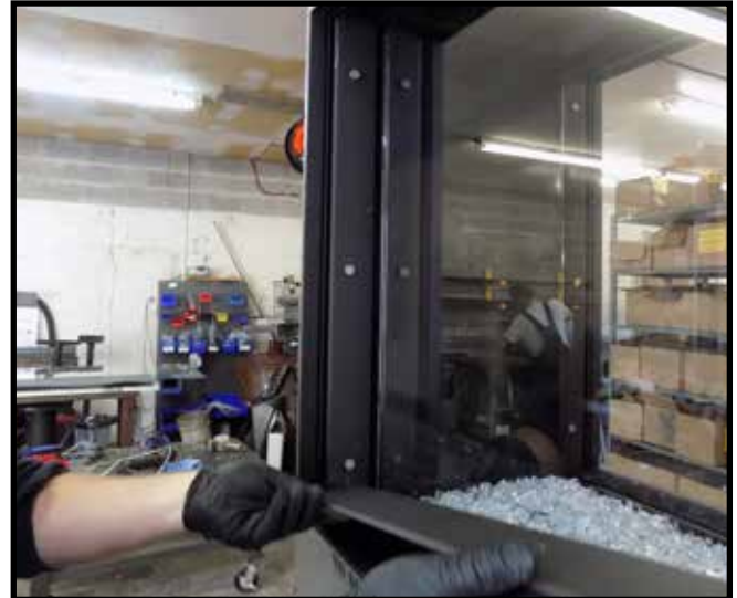
Figure 48: Insert bottom end first.
