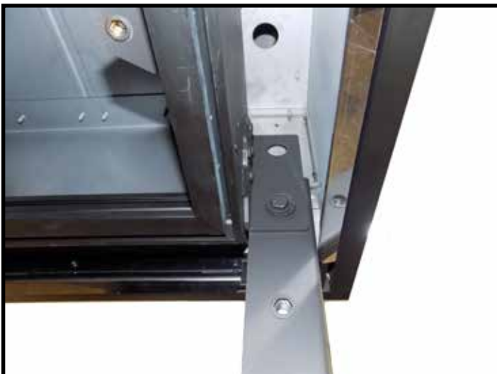
Figure 9: Vertical support upper bolt to be removed.
