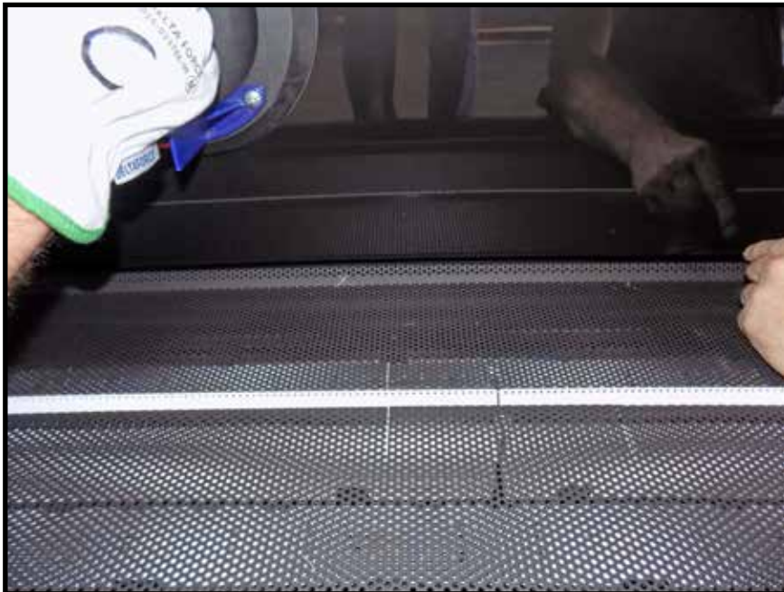
Figure 33: Lift bottom end of black glass over the rear mesh screen.
