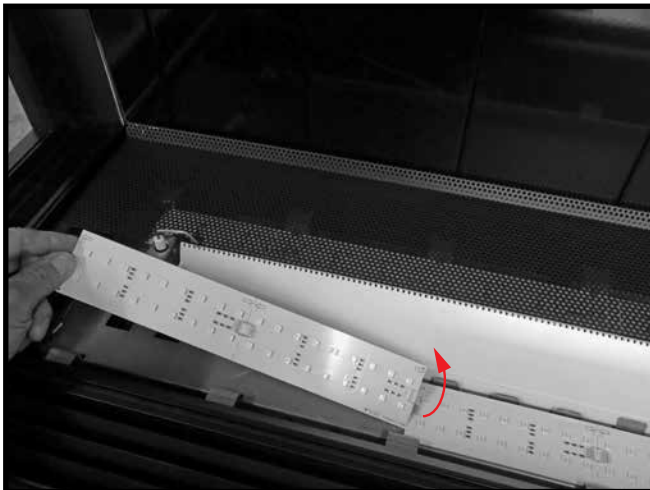
Figure 60: LED strip removal.
