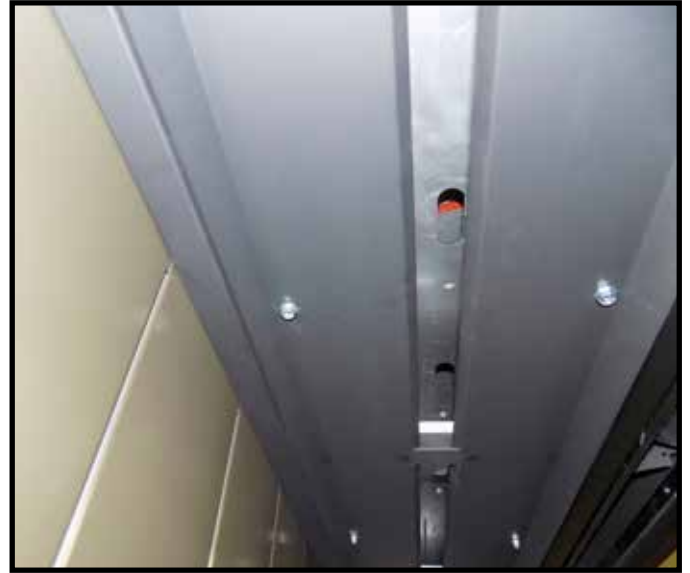
Figure 29: Adjustment accessible through the baffle cover.
