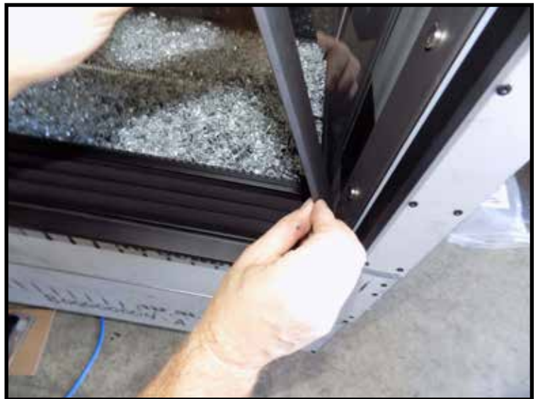
Figure 42: Installing right side securing panel.
