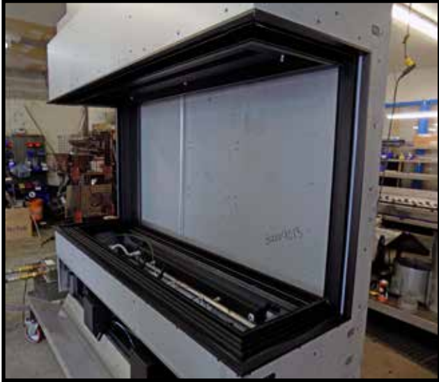
Figure 32: Rear wall before black glass sheet installation.
