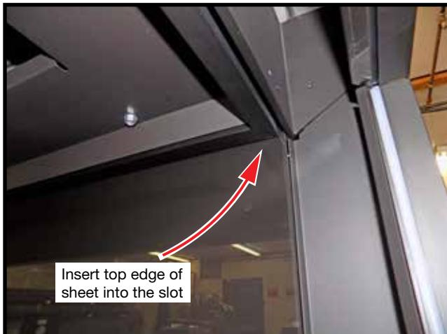
Figure 34: Inserting the top edge of sheet.
