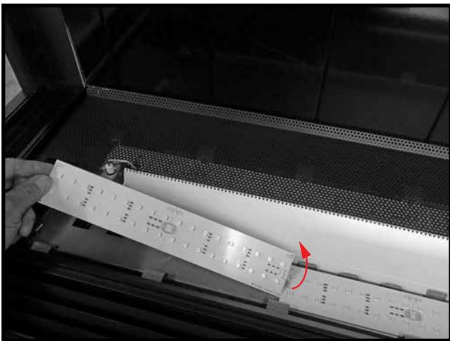
Figure 65: LED strip removal.
