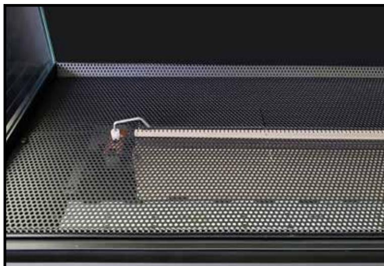
Figure 38: Burner tray in place.
