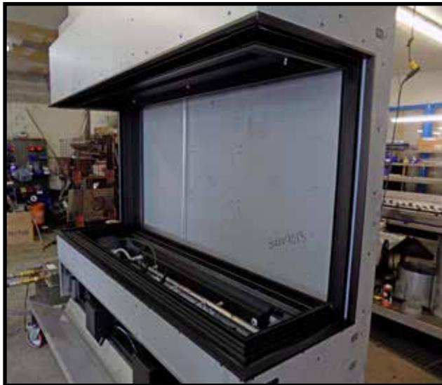
Figure 32: Rear wall before black glass sheet installation.
