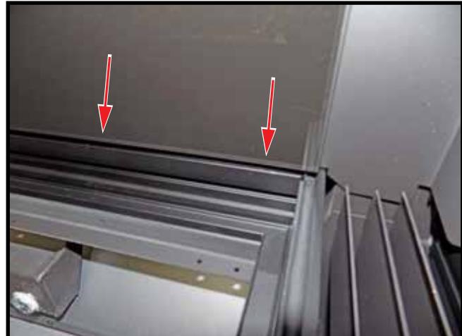
Figure 35: Lower sheet into the bottom slot.
