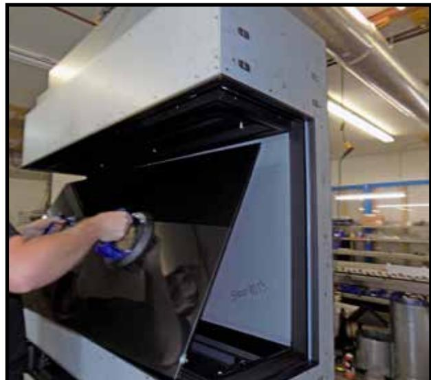
Figure 33: Insert top edge of sheet first.
