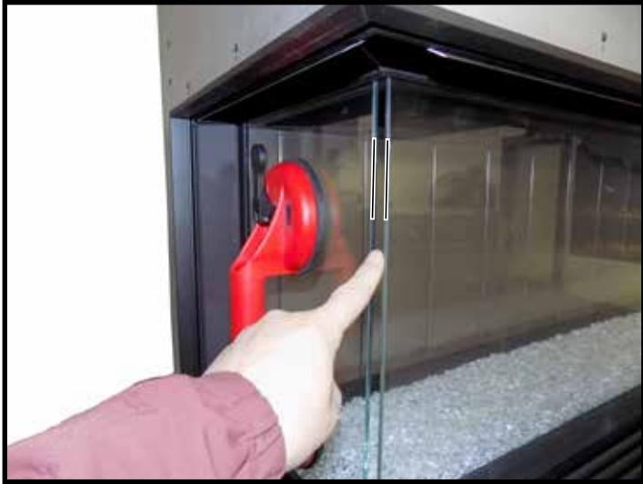
Figure 46: Gap present before sliding left side glass panel to the front.
