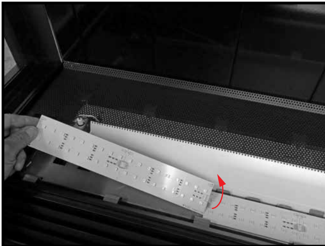
Figure 62: LED strip removal.
