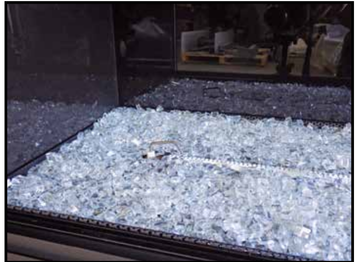
Figure 40: Crushed glass media in burner tray.
