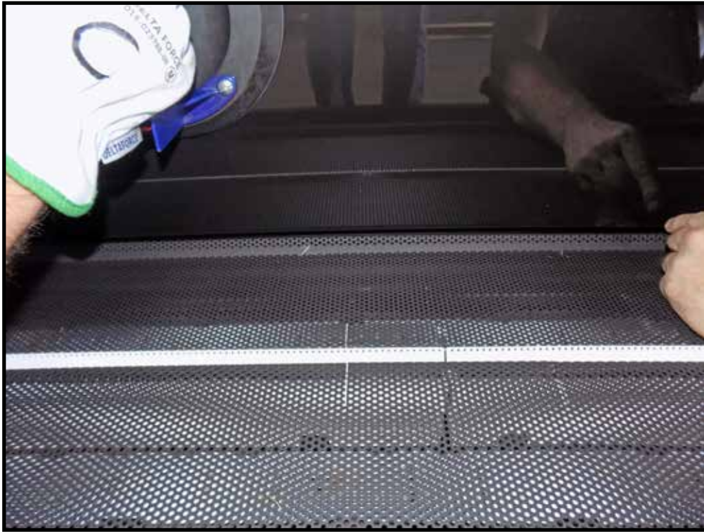
Figure 34: Lift bottom end of black glass over the rear mesh screen.
