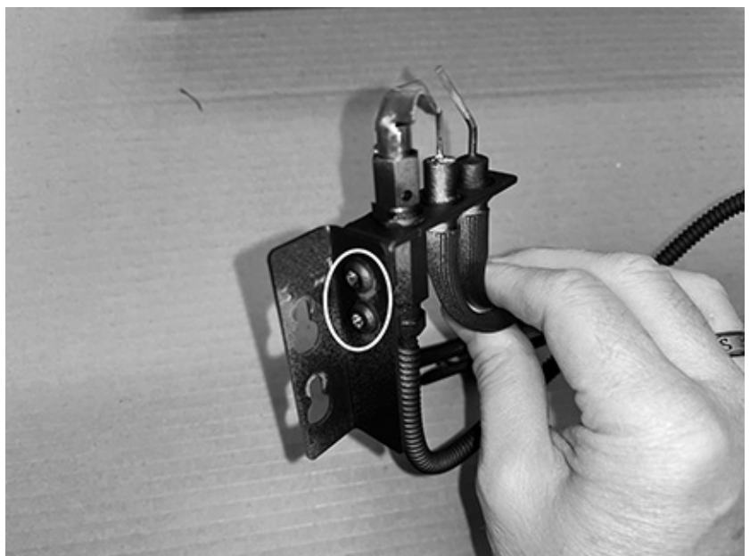
Figure 11: Remove pilot mounting bracket.
