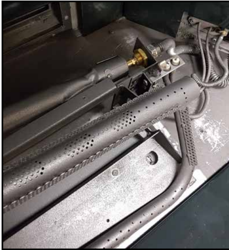
Figure 8: Securing air deflector to the burner.
