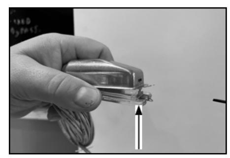
Figure 36: Push the glass lens up to close it again.
