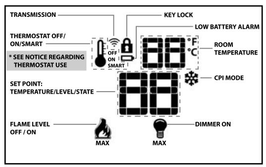
Figure 2: Proflame 2 LCD screen details.
