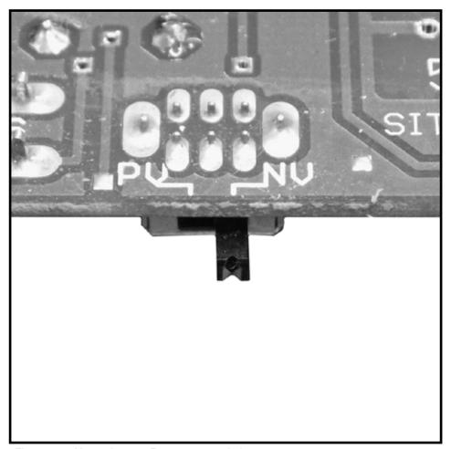
Figure 30: Natural vent - Power vent switch.
