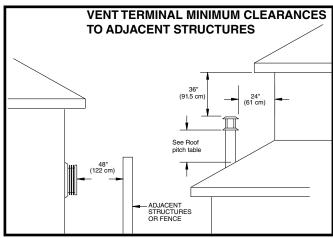
Figure 43: Vent roof clearance.
