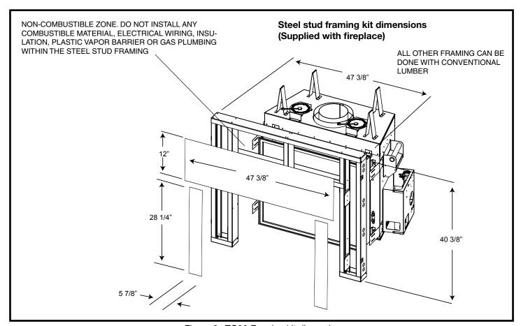
Figure 9: TC30 Framing kit dimensions.
