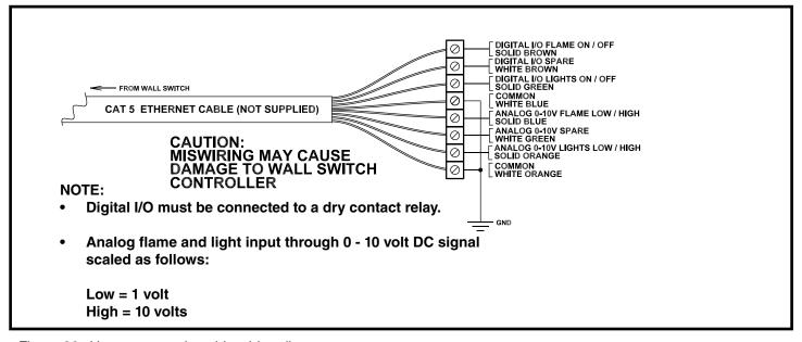
Figure 32: Home automation side wiring diagram.
