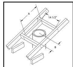
Figure 40: Roof opening for vent.
