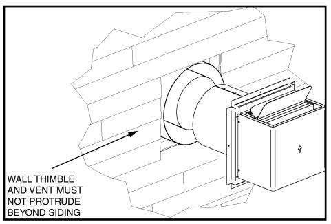
Figure 34: Wall vent terminal.
