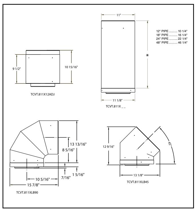
Figure 51: Vent pipe dimensions.
