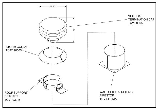
Figure 50: Roof termination kit.
