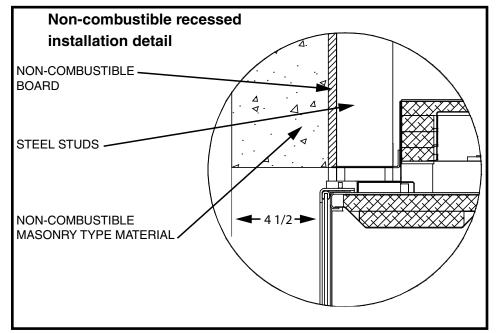
Figure 13: Recessed installation detail.
