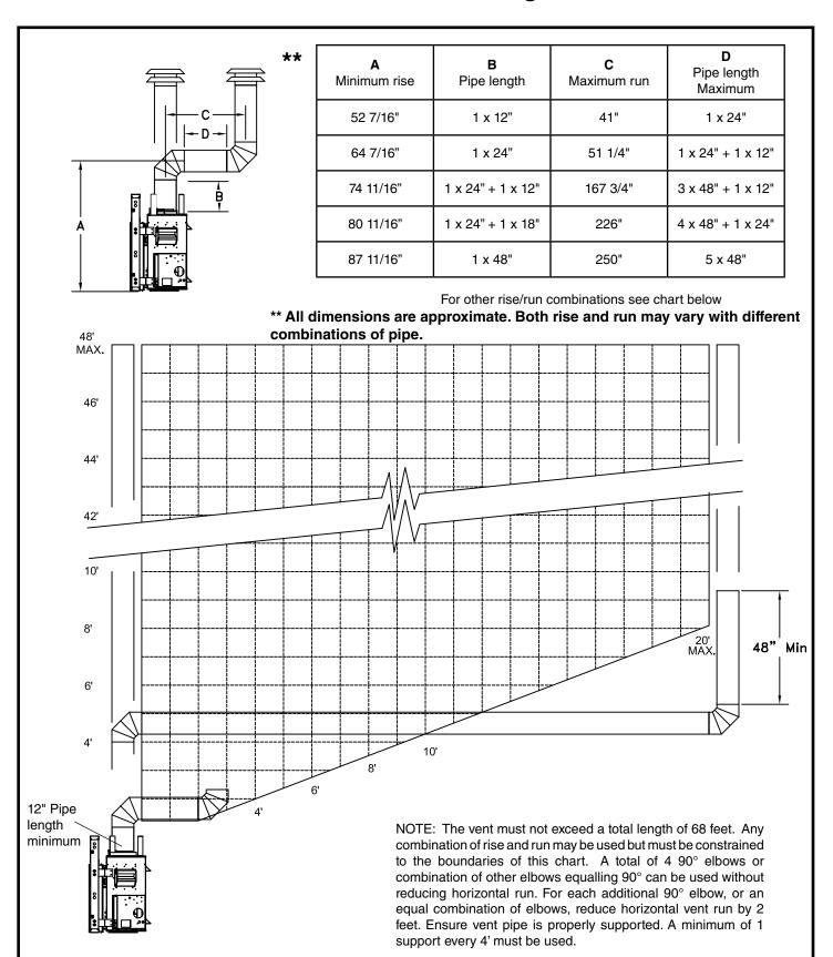
Figure 39: Roof terminal venting chart.
