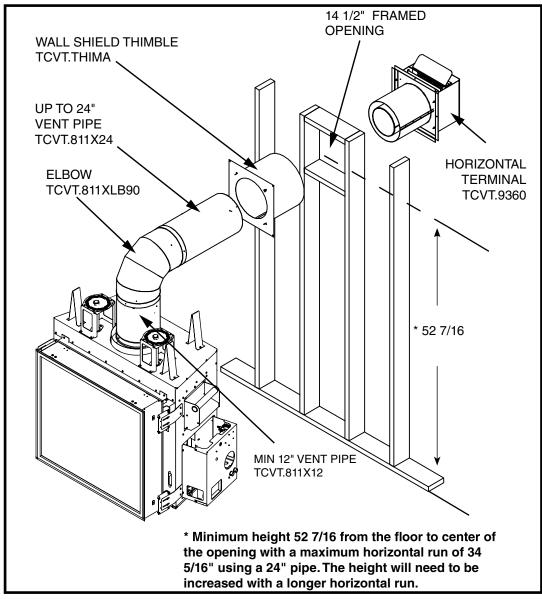
Figure 37: Wall vent terminal framing.
