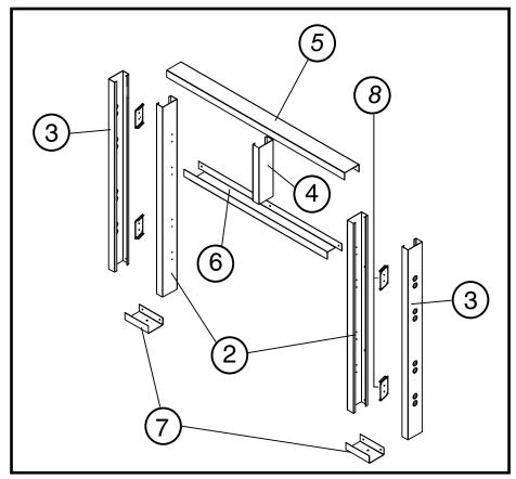
Figure 16: TC30 Framing kit parts.
