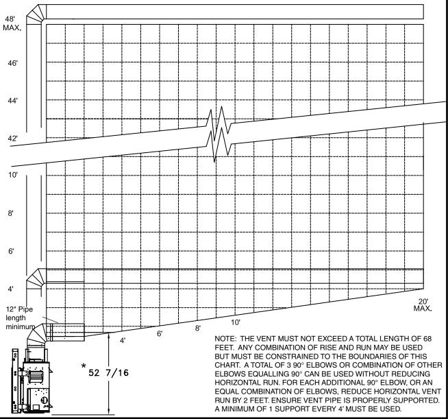
Figure 38: Wall termination venting chart.
