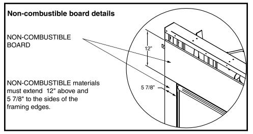
Figure 12: TC30 Non combustible board dimensions.
