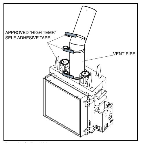
Figure 45: Sealing with tape.
