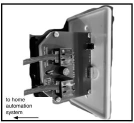
Basic Wall Switch Home Automation is limited to flame on and off using a dry contact relay with the solid brown wire and common. Figure 32.
