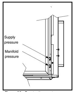
Figure 33: Gas testing ports.
