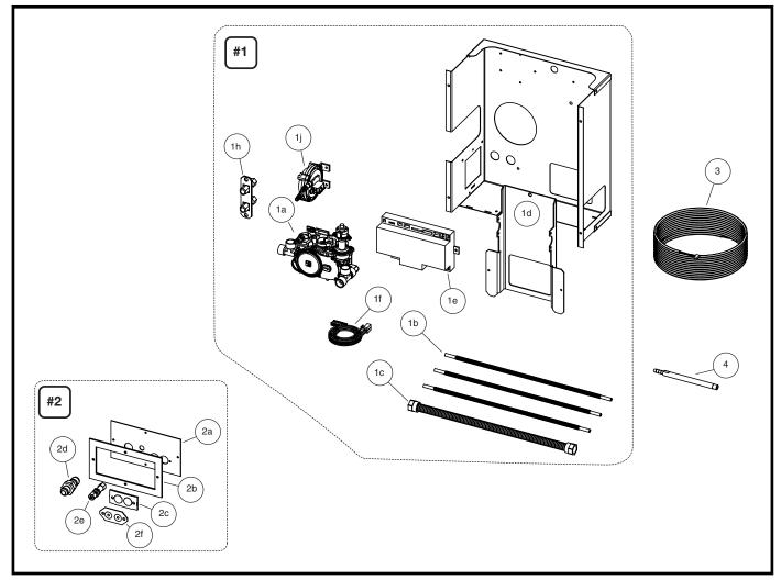
Figure 68: TC Valve control system parts. **KIT CONTENTS:**
