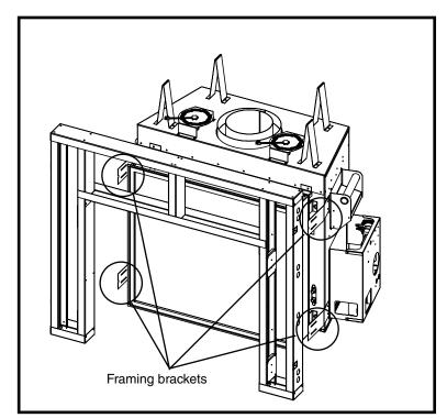
Figure 17: TC30 Framing brackets.
