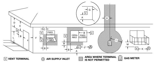
Figure 44: Vent terminal minimum clearances.
