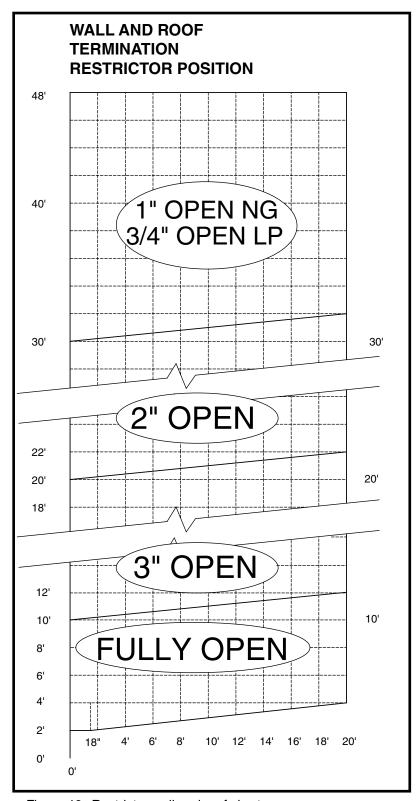
Figure 46: Restrictor wall and roof chart.
