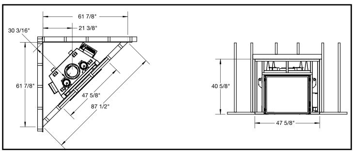
Figure 10: TC30 Minimum Combustible Framing.
