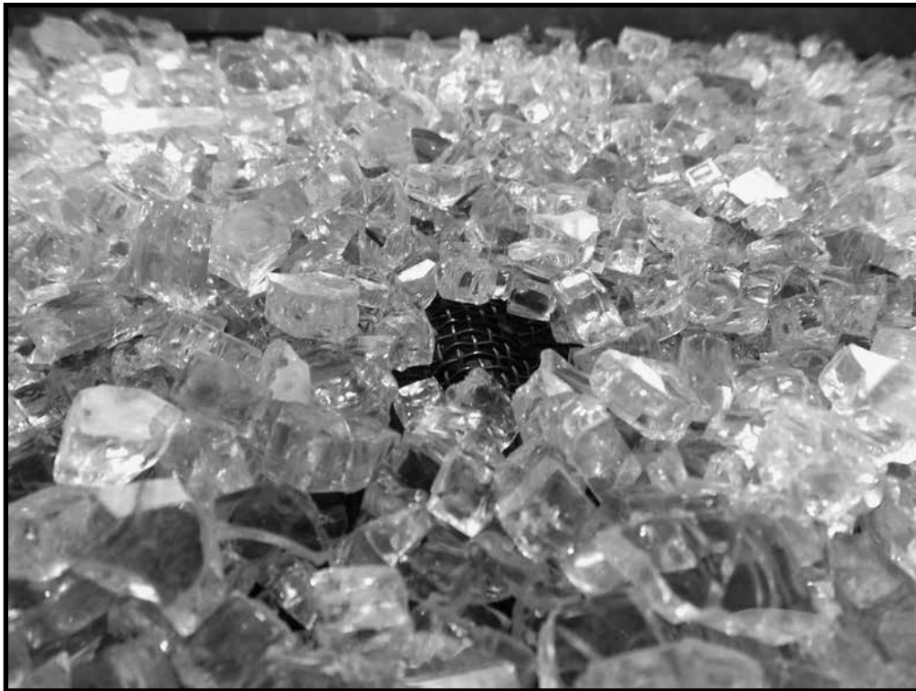
Figure 19: Bump in mesh for pilot flame.
