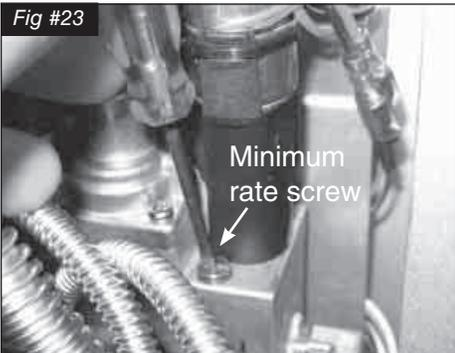
11. Remove the minimum rate screw located in the valve. (Fig. #23)
