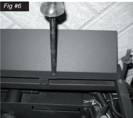
6. Attach air deflector to rear of grate with two screws (Fig. # 6)
