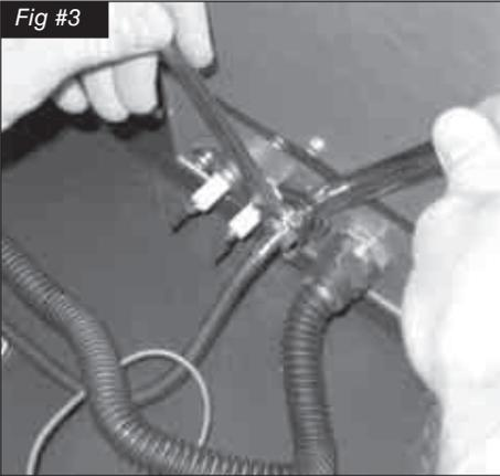
3. Attach the pilot supply tube to the bulk head fitting and tighten. (Fig. # 3)
