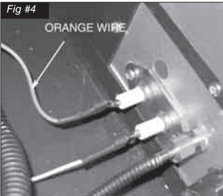
4. Connect spark electrode wire (ORANGE) to the rear electrical bulk head fitting. Connect the flame sensor wire to the front electrical bulk head fitting. (Fig. # 4)
