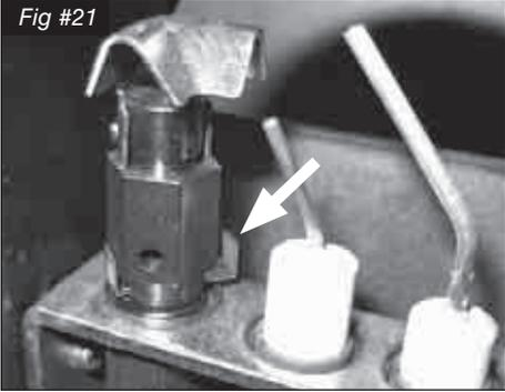
9. Slide the pilot adjustment band over and ensure that the hole in the orifice band is showing. (Fig. #21 shows NG position, Fig. # 22 shows LP position)
