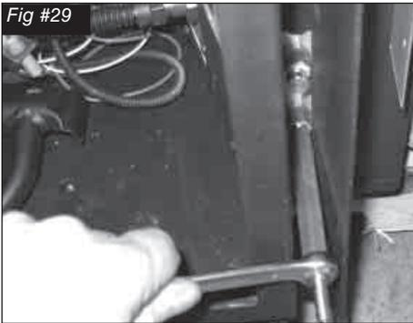
2. Thread the extension test fitting into the open test port. (Fig. #29)
