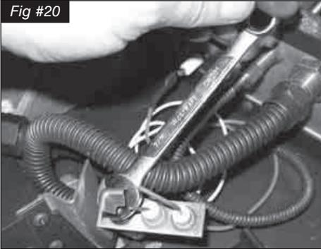
8. With a 7/16" wrench loosen the pilot head on the pilot assembly by a half-turn (Fig. #20)
