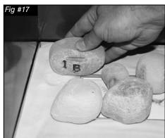
8. Repeat the sequence of placing the rocks three more times until the burner is covered.
