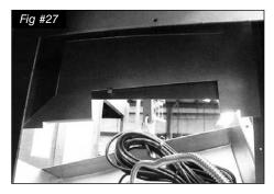
8. Lift the control box shield and rest on the edge of the screw above the access hole (Fig. #27)
