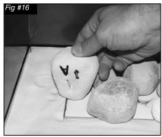
Place the two remaining rocks on the left hand end of burner as shown. (Fig. #16 and 17)
