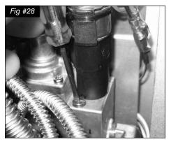
9. Remove the minimum rate screw located in the valve. (Fig. #28)
