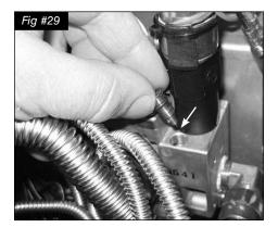
Replace the minimum rate screw with the one provided in the propane conversion kit supplied with this fireplace. Ensure that the screw is fully seated. (Fig. #29)
