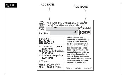
14. Fill in the date and the name of the person who performed the conversion in the white area on the conversion label. Peel off the protective backing and apply the conversion label directly over the gas specifications on the rating label.
