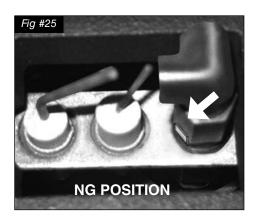
Slide the pilot adjustment band over and ensure that the hole in the orifice band is showing.
