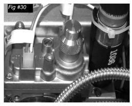
Remove the aluminum cap from the top of the pressure regulator. (Fig. #30)
