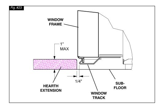
Caution: While a hearth extension is not required and combustible flooring materials may be brought directly up to the fireplace, many materials (such as wood flooring) may not tolerate the radiant heat from this fireplace, resulting in discoloration, shrinking and cracking. For this reason, we suggest a non-combustible hearth that is no more than 1" above the bottom of the fireplace. If thicker, fireplace must be raised accordingly.
