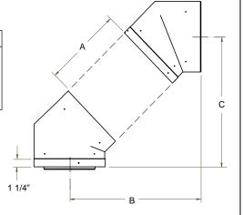
ADDING AN ADJUSTABLE SECTION TO PIPE WILL INCREASE OFFSET BY 2 1/8" TO 6 3/4"
