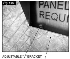
The lower rear panel is held tight against the side panels by two "V" brackets located on the firebox rear wall. Although the brackets are adjusted at the factory for the best fit, some adjustment may be necessary. Adjust the angle of the bracket by hand to ensure a snug fit.
