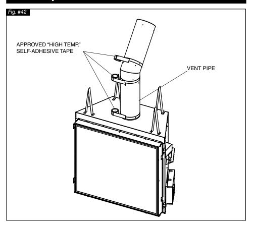
All outer joints of the vent pipe must be sealed with the approved "High Temperature" self-adhesive aluminium tape provided. Wrap the tape completely around the joint and press firmly in place.
