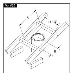
Size of the opening will have to increase with the pitch of the roof to ensure a 1 3/4" inch air space clearance between vent pipe and combustibles.
